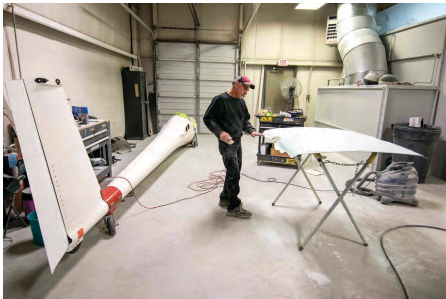
Joseph DeRosa sands a fiberglass belly pan of an aircraft that is under repair at SouthTecAviation, an aviation repair facility at Mid-Carolina Regional Airport.
