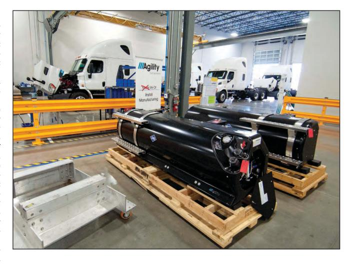
Above: A pair of Compressed Natural Gas saddle tanks at Agility Fuel Systems that will go on a tractor-trailer.
