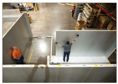
One of the final steps in the manufacturing of the walk-in coolers produced by Imperial Brown is to set up the panels and doublecheck for quality assurance. Chad Archer (right) pieces together a larger project.
