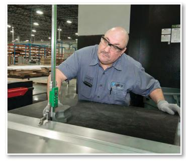
On the cover: Geoffrey Ellis checks the height of a sheet of formed aluminum to make sure it meets the correct specifications at Agility Fuel Systems. The facility builds Compressed Natural Gas fuel cells for tractor-trailer engines. — Photo by Jon C. Lakey.
